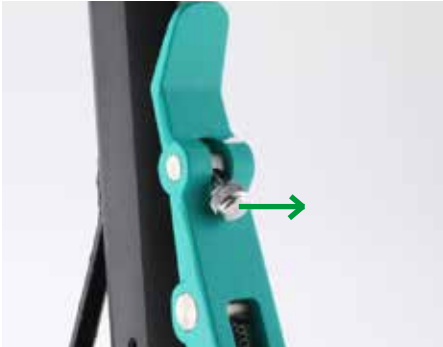
1 Loosen the safety screw
