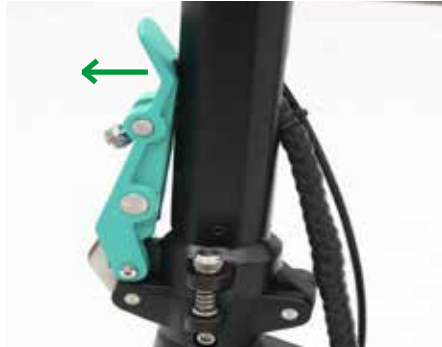
2 Plate opening and folding buckle
