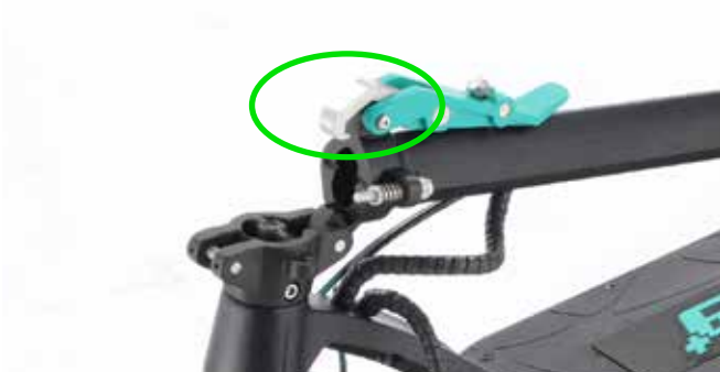
4 Once the main lever is released, ensure that the capture is also released
