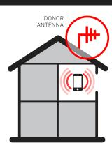
Install **Donor Antenna** where the mobile device receives this signal.
