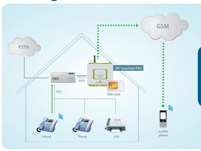
In this scenario, companies connect the  $2N^{\circ}$  EasyGate PRO to their existing PBX with an analogue interface. All calls to mobile networks are routed via the gateway and customers can save up to 70 percent on their calling costs.
