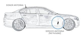
Install Service Antenna in the cab, towards the front, where coverage is needed. Ideally, there should be substantial material, like the metal of the roof, between the Donor and Service Antennas, to improve isolation.
