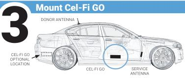
Find a good mounting location in your vehicle. Location should have airflow and be secure from contact with external objects.
